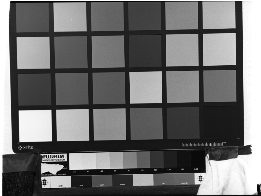
Normal ID-11 development. Negative scanned at 4000 dpi with Nikon Coolscan 9000ED without digital processing.
